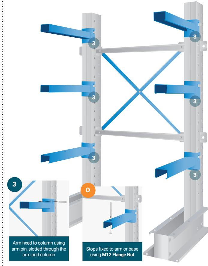
**1A** Position the column alongside the four fixing holes on the side of the right and left floor bases. To do this you will need to lift the column slightly off of the ground. Once aligned, fix the floor base to the column using **4 x M10x130 Bolts, 4 x M10 Washers and 4 x M10 Flange Nuts**.
